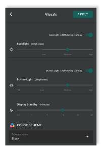
The back-light of the rotary encoder dial can also be deactivated when the display is in standby mode, within the settings menu of the Zone Controller itself.
