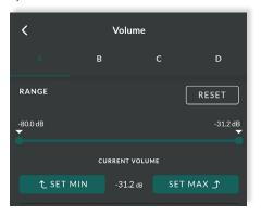
On the device, the end user is made visually aware of the volume range limitation when adjusting the volume level (see below).
