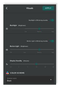
The intensity of the back-light behind the rotary encoder dial can also be customized within the settings menu of the Zone Controller itself. To change the intensity of the backlight behind the rotary encoder dial via the Zone Controller, simply follow the steps outlined below.
