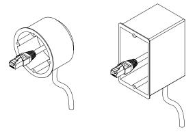
3. Connect the Ethernet cable to the Zone Controller unit.
