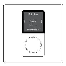
3. Tap the rotary encoder to confirm the selection of the option labeled "Static".
