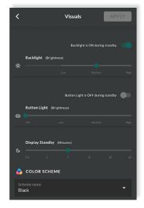
The intensity of the display screen's back-light can also be customized within the settings menu of the Zone Controller itself. To change the intensity of the display screen's backlight via the Zone Controller, follow the steps outlined below.
