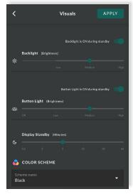
The display screen can also be deactivated when the display is in standby mode within the settings menu of the Zone Controller itself.
